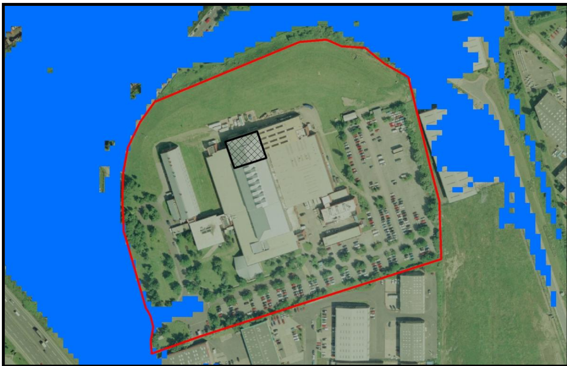
Mapping of the predicted flood extent for the study site using GIS.
